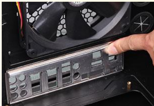
Installing the shield
