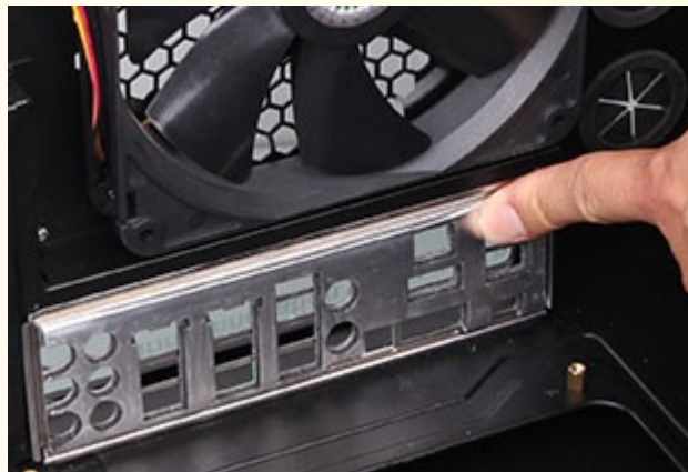
Installing the shield
