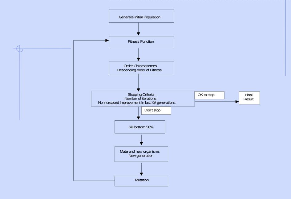
Figure 1 Typical Genetic Algorithm Block Diagram
